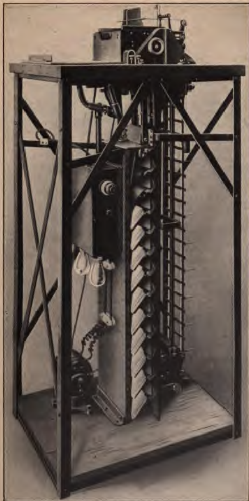
DIAGRAM 14. HOLLERITH SORTING MACHINE FOR CLASSIFYING SCHOOL STATISTICS
